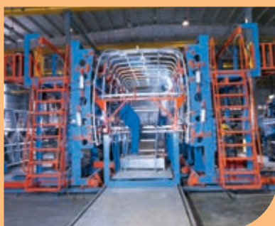
Jigs and fixtures for controlled dimensions and perfect alignment
