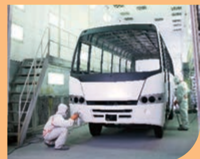
Rigid and strong tubular bus construction, integrated with chassis
