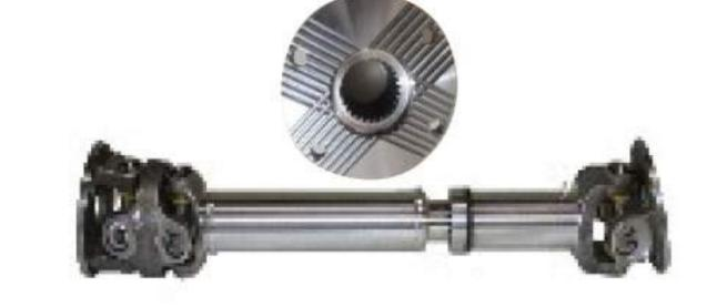
Serrated Coupling flange propeller shaft for better Reliability, Maintenance & to increase Power Transmission
