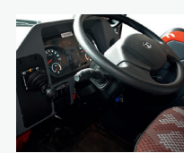
Tilt and telescopic Power Steering- Adjustable to any driver with respect to his height
