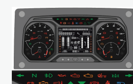
New Multifunction Instrument Cluster Features: Average Fuel Economy, Trip A&B Gear Shift Advisor, Driver massage screen Tell Tale Symbols
